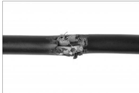
Damaged electric cable
